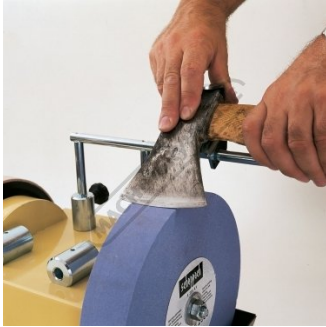
Jig 40 is the perfect attachment for axes with a blade up to 170mm
