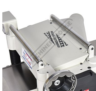
Top Rollers for Returning Material
