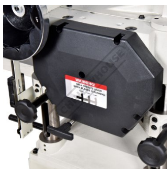
2 Speed Feed Gearbox
