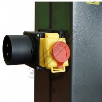
Electrical Emergency Stop
