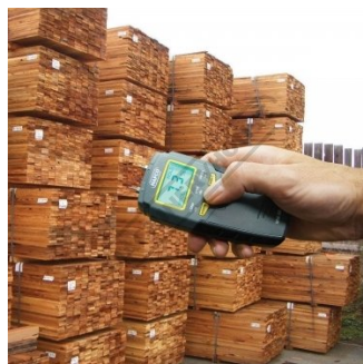
Measuring Moisture Content in Wood
