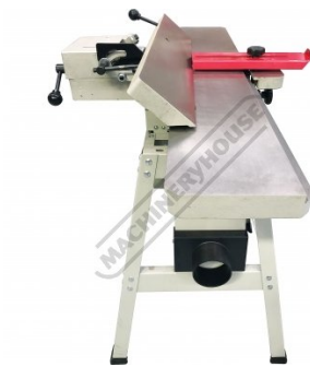
Tilting Fence to 45 Degrees
