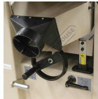
Dust Chute Set Up For Planer
