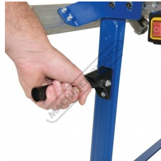
Handles For Moving Saw Around
