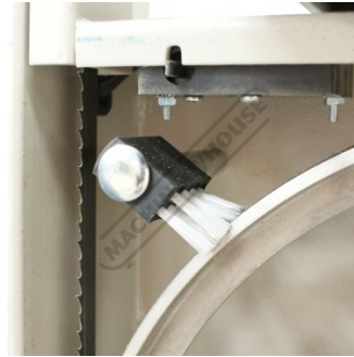
Blade Brush and Safety Guard Micro
