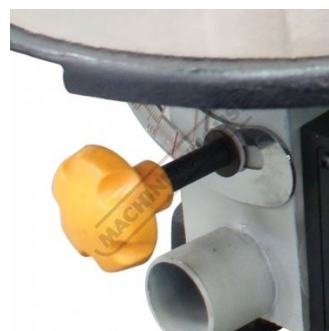
Cast iron table tilts 45degrees to the left and 8degrees to the right
