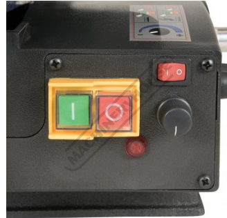
On Off Switch & Variable Blade Speed Dial
