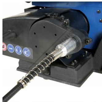
Drive Connector For Flexible Shaft Attachment
