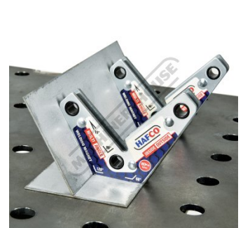
Mult Angle Magnet Shown Setup in 120 Degrees
