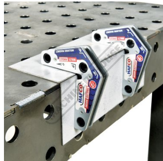
Mult Angle Magnet Shown Setup in 90 Degrees
