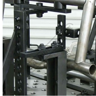
Use Ball Lock Bolts to fasten elements to the tabletop or to economy clamping squares or right angle brackets
