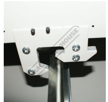
Drawer in Unlock Position
