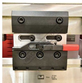
Quick Release Tool Clamps Change Tools Without Sliding Them All Out
