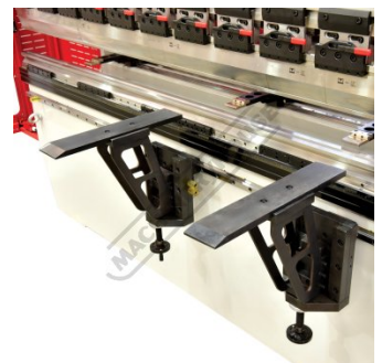
Adjustable Sliding Front Sheet Supports
