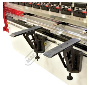
Adjustable Sliding Front Sheet Supports
