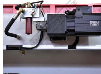
Eco Friendly Servo Driven Hydraulics
