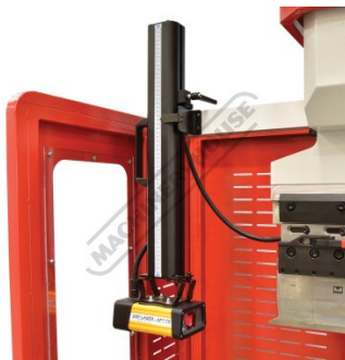
Laser Guarding System With Alignment Guide
