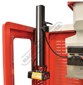
Laser Guarding System With Alignment Guide
