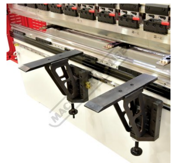
Adjustable Sliding Front Sheet Supports
