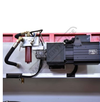
Energy Saving Servo Driven Hydraulics
