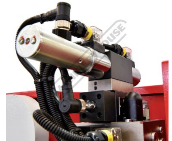
Safety Hydraulic Monitoring Valve
