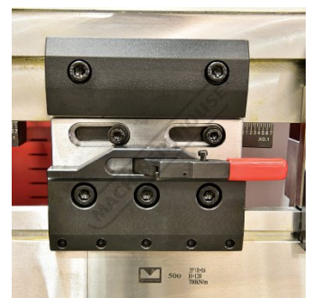
Quick Release Tool Clamps Change Tools Without Sliding Them All Out
