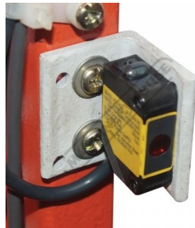
Safety Omron E3ZS Rear Light Sensor Guarding
