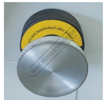
Fine Adjustment Dial for Backgauge
