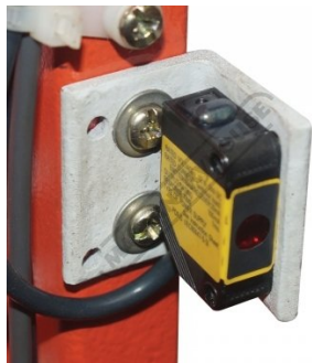
Safety Omron E3ZS Rear Light Sensor Guarding
