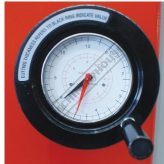
Variable Blade Gap Adjustment Dial
