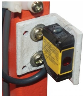
Safety Omron E3ZS Rear Light Sensor Guarding
