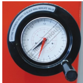
Variable Blade Gap Adjustment Dial
