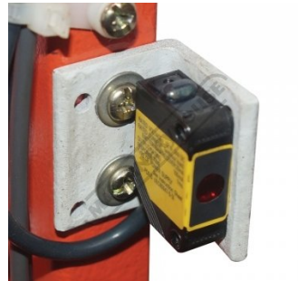
Safety Omron E3ZS Rear Light Sensor Guarding
