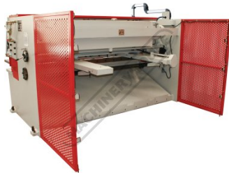
Rear guarding with safety sensors
