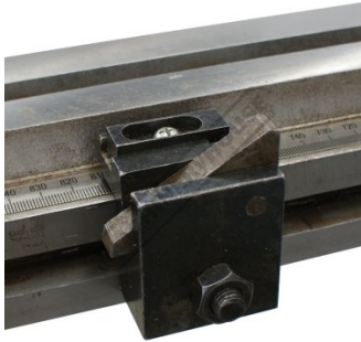
Flip over material stop
