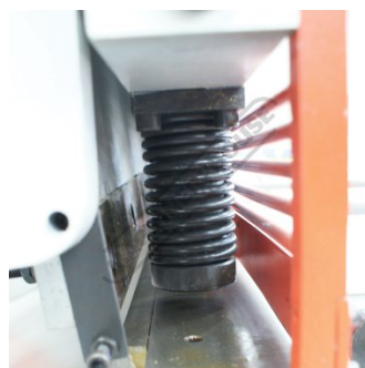
Hydraulic material hold downs
