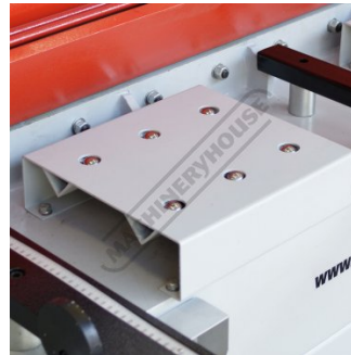
Material Transfer Balls on the Table
