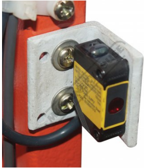
Safety Omron E3ZS Rear Light Sensor Guarding
