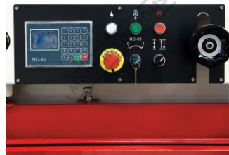
NC 89 Control Panel
