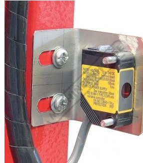
Safety Omron E3ZS Rear Light Sensor Guarding
