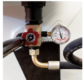
Return Tank Pressure Gauge
