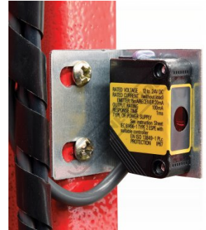
Omron E3ZS Rear Light Safety Guarding Sensor
