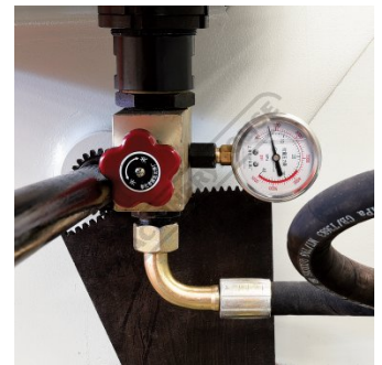
Return Tank Pressure Gauge
