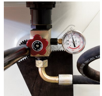
Return Tank Pressure Gauge
