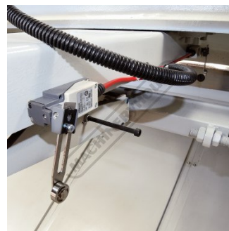
Backgauge Limit Trip Switches
