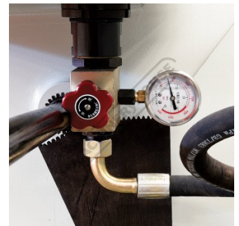
Return Tank Pressure Gauge
