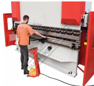
Laser Guarding system In Use
