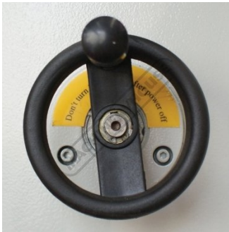
Fine Adjustment Beam Positioning
