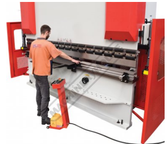
Laser Guarding system In Use
