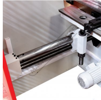
Estun NC E21 Control Ballscrew Backgauge
