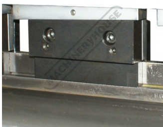
Adjustable Top Tool Taper Wedge System
