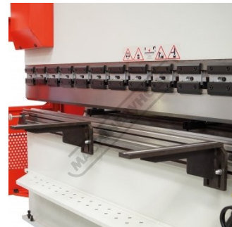
Adjustable and Sliding Front Sheet Supports
