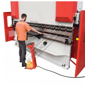
Laser Guarding system In Use
