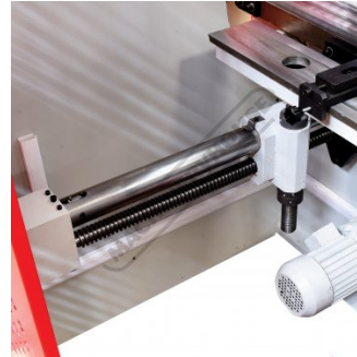
Estun NC E21 Control Ballscrew Backgauge
