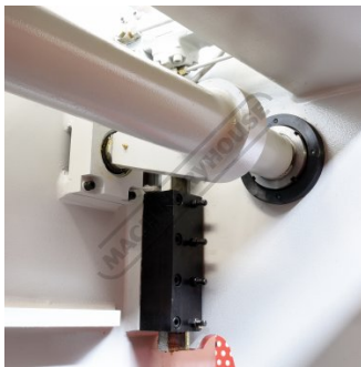
Synchronised Torsion Bar
