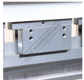
Adjustable Top Tool Taper Wedge System
