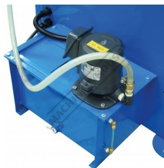
Coolant Pump and Tank
