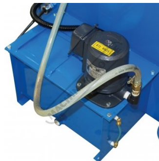
Coolant Pump and Tank
