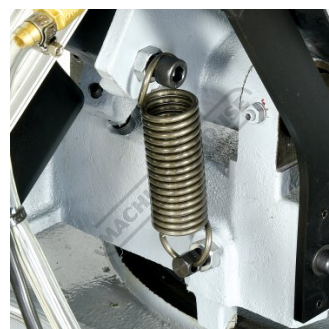
Spring Assisted Head Return
