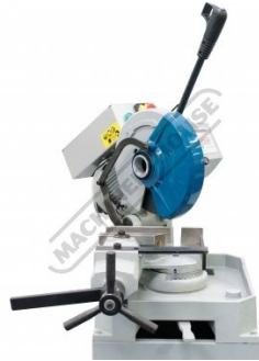
Swivel Head to 45 degrees in Both Directions
