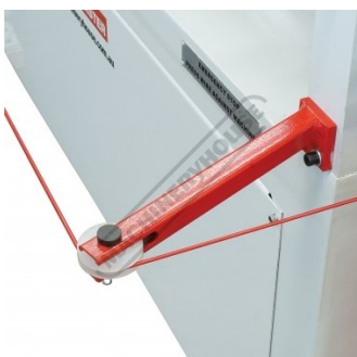
Safety Wire Interlock System
