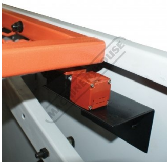
Safety Micro Switch on Rear Gate
